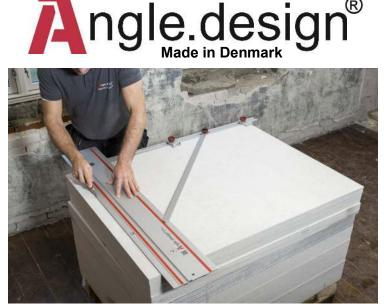
**2.** When cutting with a blade knife, turn the guide rail over to use the other side. The measurements remain valid even when the guide rail has been turned over.
