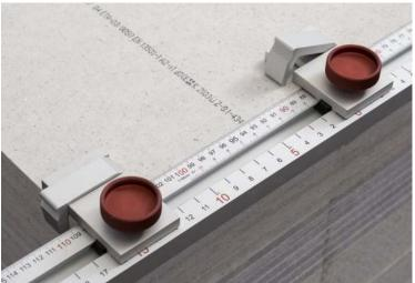
**8.** The end stopper grips the board and maintains its position relative to the ruler measurement. When not in use, the end stopper can simply rest on the board. The end stopper is also useful when using an extension, as it supports the main rail.
