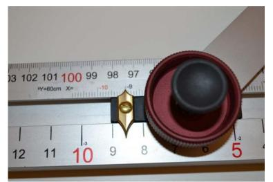
**7.** The small "Y = 60 cm" scale may be used for boards out of angle. Here, the small arrow is pointing to -9. On this setting, the board will be cut 9 cm out of angle on a 60 cm board. For a 120 cm board, the cut will be 18 cm out of angle.
