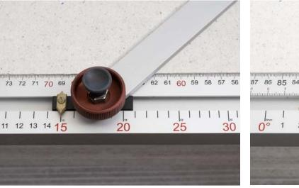
**5.** Note that when the angle is changed from 90°, measurements on the main rail are distorted. The size of the distortion is indicated above the angle. For example, the image shows an angle of 15°. Above the angle, a small "10" indicates that the desired dimension for the cut has been lengthened by 10 mm.
