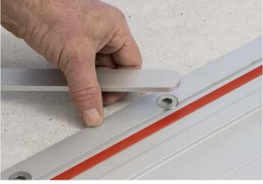
**8.** When the diagonal strut must be removed, apply downward pressure with your thumb while lifting with the fingers so that the lock pops up.
