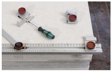
4. With the main rail turned as in figure 3, if you still wish to use the end stoppers, the attachment on the sliding bracket must be reversed. Loosening the set screw allows you to remove the attachment, so you can reattach it to the other side of the sliding bracket.
