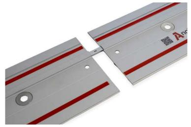
**11.** If the guide rail must be extended, insert the fitting into the groove in the rail. Then, bring the ends together and tighten the set screws on the underside of the fitting.
