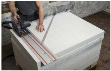
**1.** The Angle.Design angle set is shown here in use with a track saw. The guide rail is suitable for all plunge saws.
