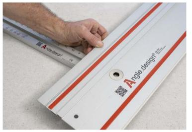
**10.** When disassembling the guide rail, place it on a hard surface before separating the units. Apply pressure to the main rail with the base of the hand. Then, lift the guide rail with the fingers until the parts are separated.
