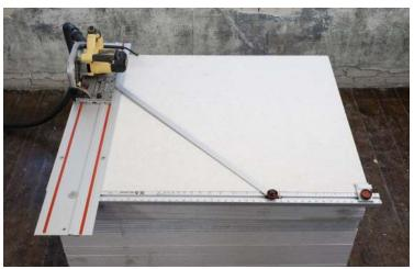
**3.** When sawing boards on the left, turn the main rail as shown in the photo. Note that in this case, measurements and angles must be read upside down.
